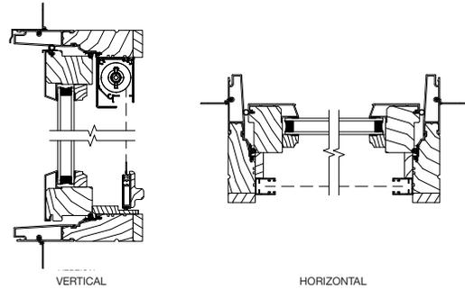
**Triple IG Casement Push-out with Retractable Screen**
