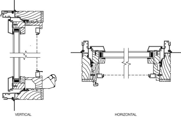
**Pinnacle Clad Awning with 3-1/4" Frame – Operating**
