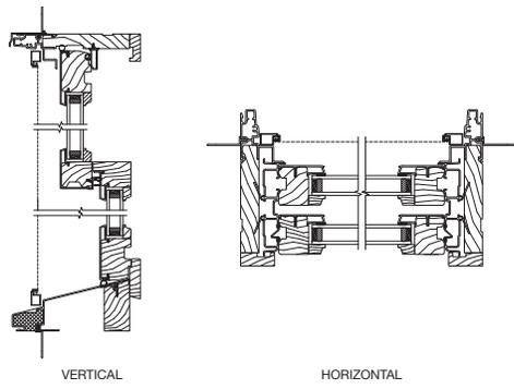
**Pinnacle Clad Concealed Jambliner Double Hung - Operating**
