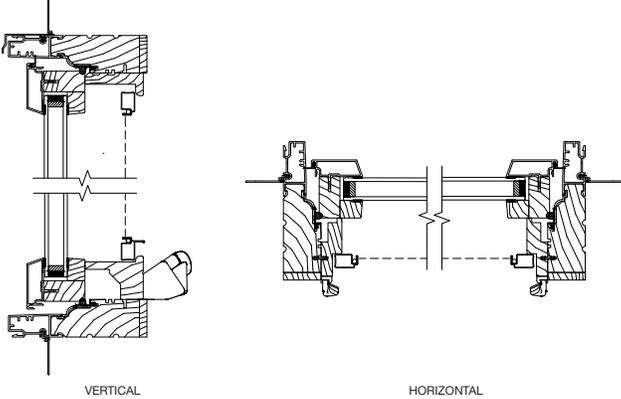
**Pinnacle Clad Casement with 3-1/4" Frame – Stationary**
