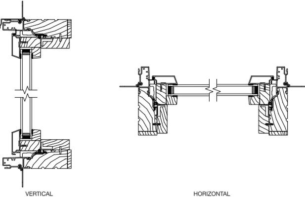
**Pinnacle Clad Awning with 3-1/4" Frame – Stationary**
